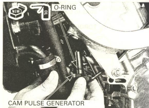
Install and tighten the mounting bolt securely.
