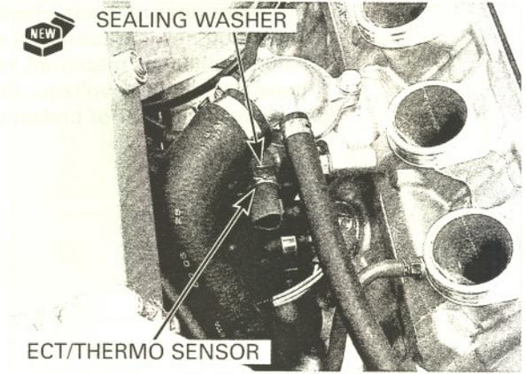
Connect the ECT/thermo sensor connector.
