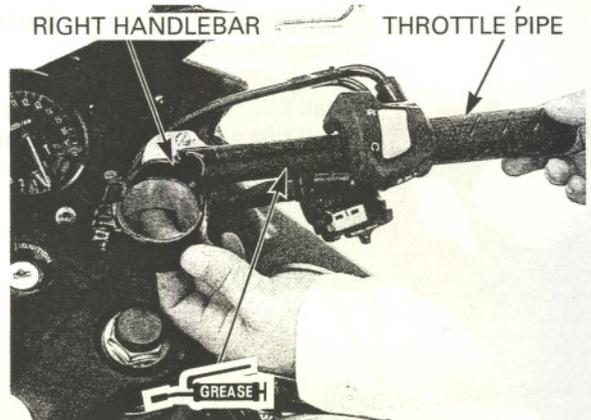
Install the each handlebar onto the fork tube, aligning its boss with the groove in the fork top bridge.
