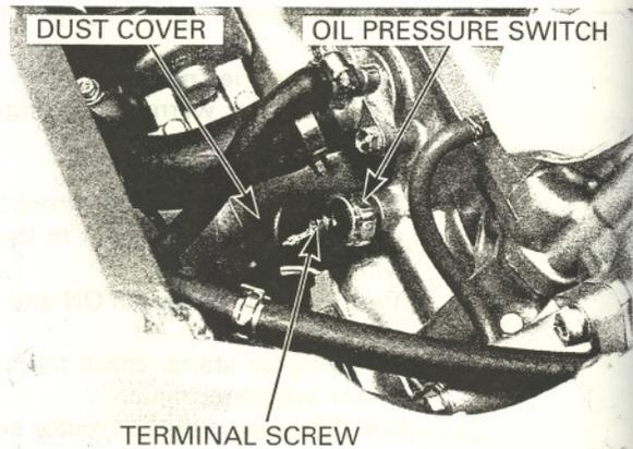
Short the oil pressure switch wire terminal with the ground using a jumper wire. The oil pressure warning indicator comes on with the ignition switch is ON. If the light does not come on, check the sub-fuse (10A) and wires for a loose connection or an open circuit.
