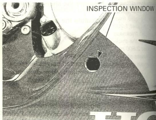
If the level is below the lower line, remove the oil filler cap and fill the crankcase with recommended oil up to the upper level line.
