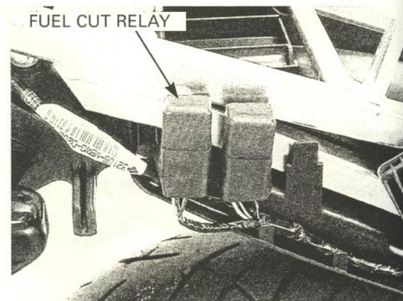
Connect the ohmmeter to the fuel cut relay connector terminals.
