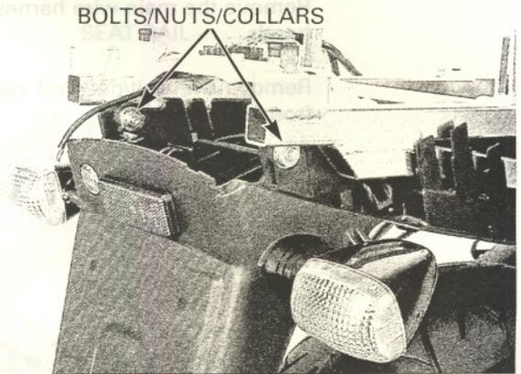
Route the rear sub-harness properly and install it into the rear fender wire guides. Install the fuel cut relay and engine stop relay onto the rear fender bosses.
