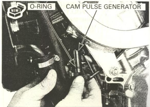
Install and tighten the mounting bolt securely.
