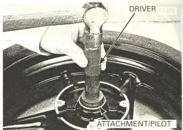
Press the driven flange collar in the new driven flange bearing until it is fully seated.
