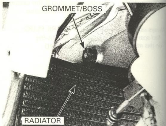
Install the washer and radiator upper mounting bolt, then tighten the bolt.
