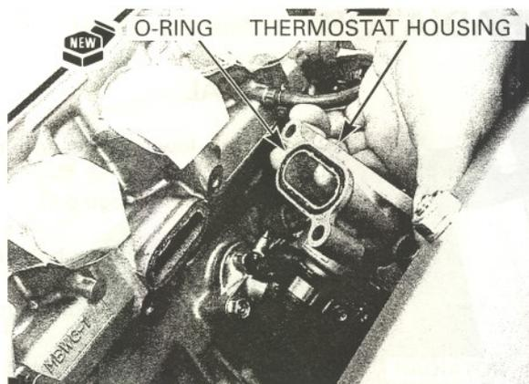
Install and tighten the thermostat housing mounting bolts.
