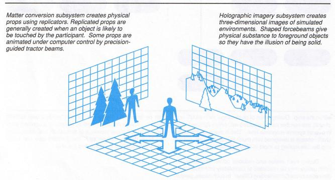
Substrate forcefield creates "treadmill" effect, permitting participant to remain stationary while the simulated environment "scrolls" by, within the limits of the simulation program.
